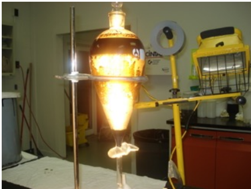
Picture 2: Oil-water emulsion after treatment.
