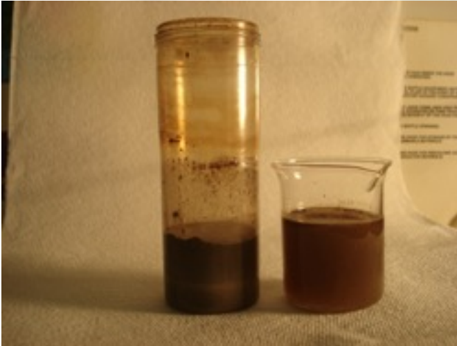
Picture 6: Left vial shows sediment; right beaker shows removed water with some sediment remaining.
