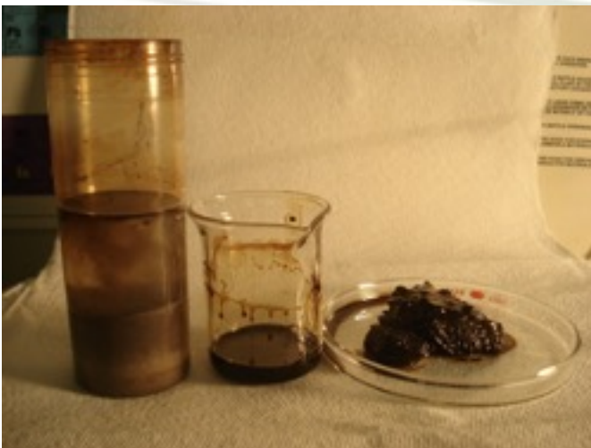
Picture 4: Left to right, water and sediment, oil, and bituminous clay after separation and removal.
