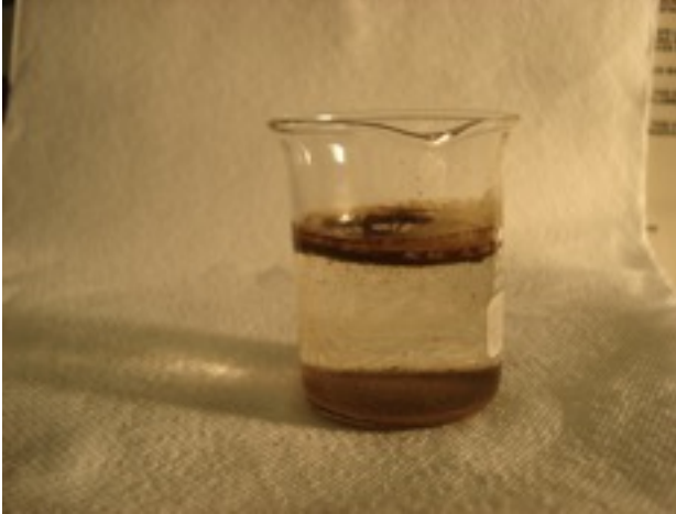
Picture 8: Separated water after 1-day of additional settling.
